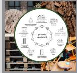
The concept of producing ecological furniture boards is to use wood-based materials that have already been used, such as old furniture, wooden chairs or pallets, so there is no need to cut down new trees. The entire board production process is an integrated and repeatable cycle, from collecting waste wood to recycling and transforming raw materials into a new and functional product.
