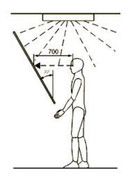
Panel evaluation should take place under a diffuse and fixed light source that illuminates the surface uniformly. This can be sunlight or adequate artificial lighting (between 2000-5000 lux). The approximate distance between the assessed surface and light source should be 1,5m. Surface defects will only be acknowledged if they are larger than 0,8mm<sup>2</sup> and visible from a distance of 0,7m at a viewing angle of approximately 45°.
